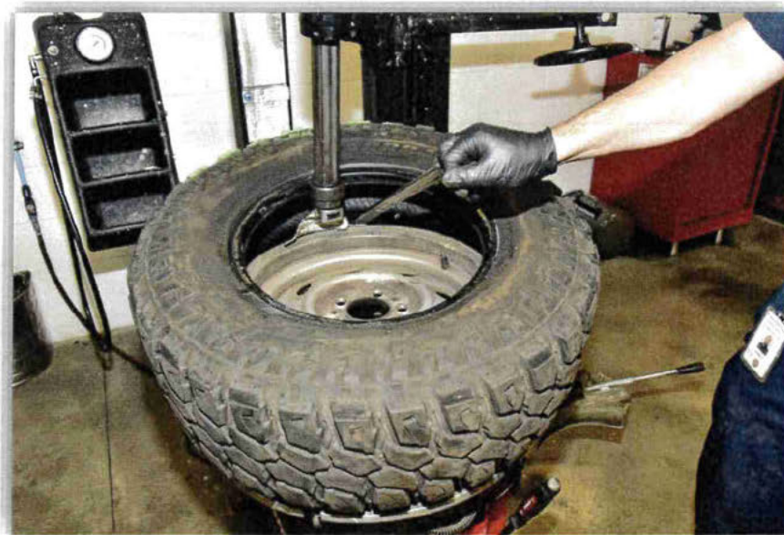
Figure 3 MMG_0059 Removal of the tire from the rim
